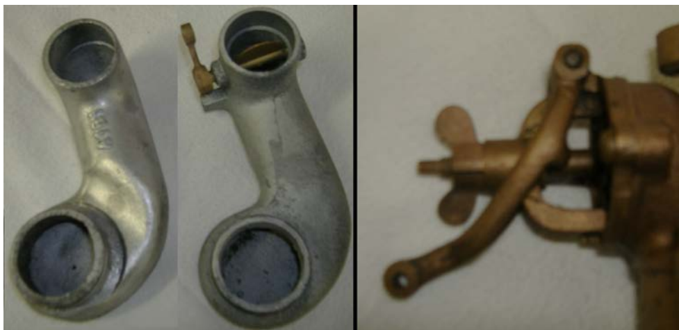
Photo # 3 showing the early (Left) and late (right) choke assembly.
