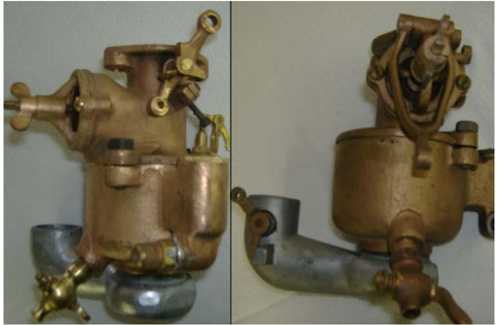
Photo # 1 (Left) showing early carburetor and Photo # 2 (Right) showing late carburetor.
