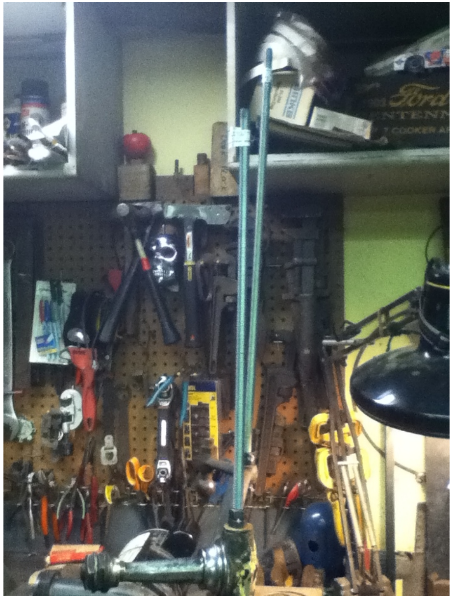
Alignment tool installed in one of my E-M-F Spindles quickly shows an alignment problem between the Kingpin and the Tie-Rod end connection.
