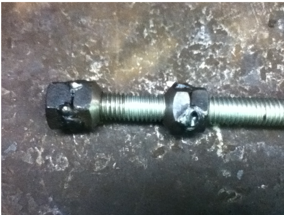
This picture shows the basic tool I made to check the alignment of my spindles.
