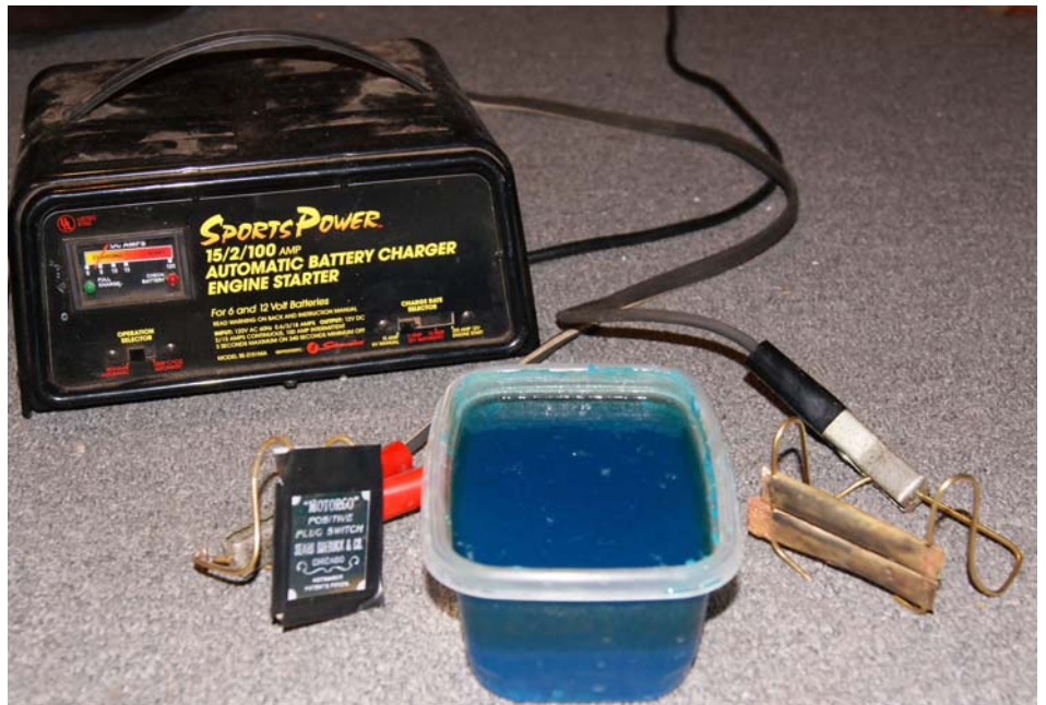
Set up showing Battery charger, piece to etch connected to Anode terminal and negative terminal attached to cathode, and the tank with Copper Sulfate solution.
